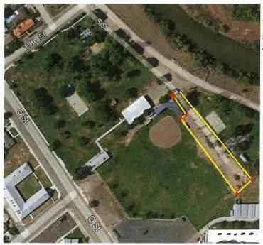
Note: The proposed work includes paving the existing lot at the end of S Street perpedicular to 16th Street adjacent to the Dunkle Park. The lot measures 450'x65' for an area of 29,250 SF.
