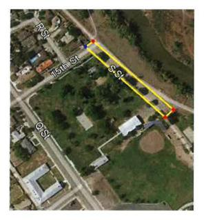
Note: The proposed work includes paving S Street from 15th Street. The street measures 545'x36' for an area of 19,620 SF.
